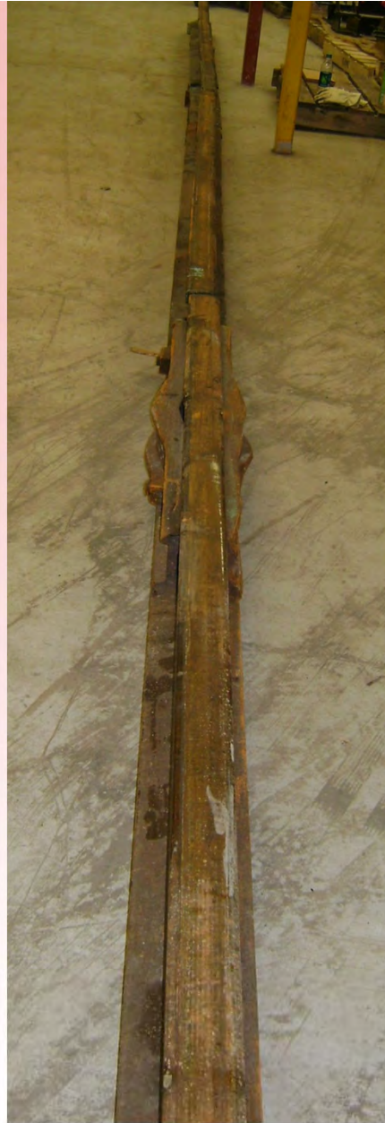
Broken rail assembly (samples 15 and 16)
